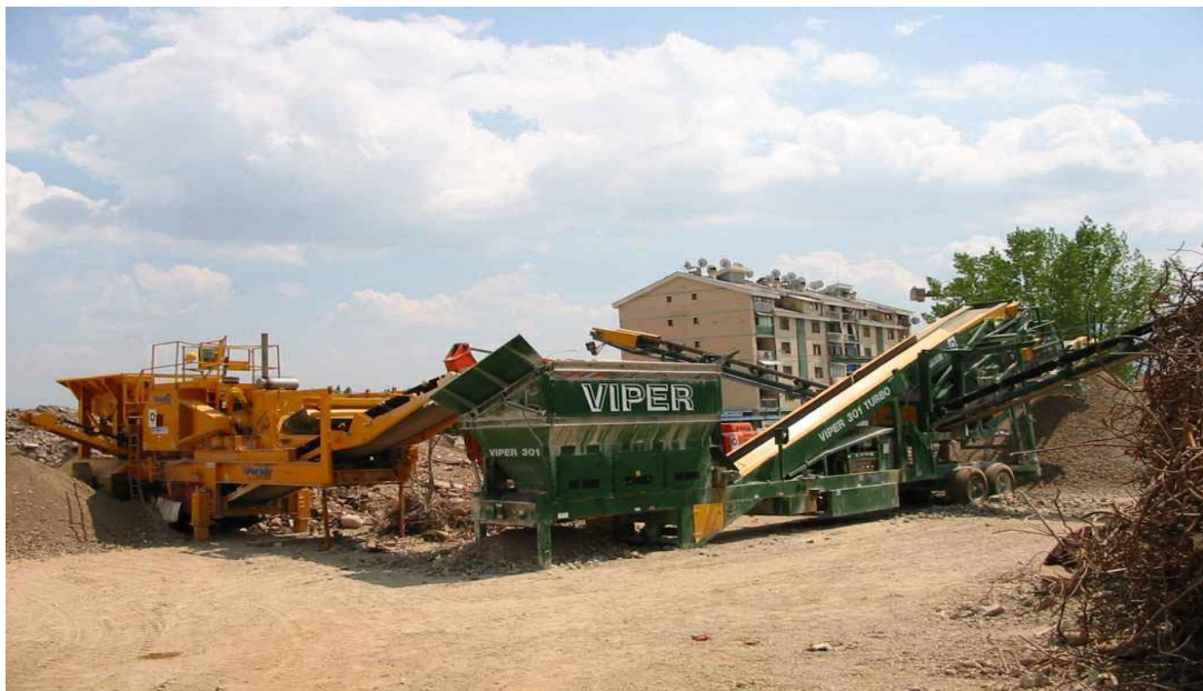
Photograph 4. Recycling plant for demolition wastes in central Kosovo.
